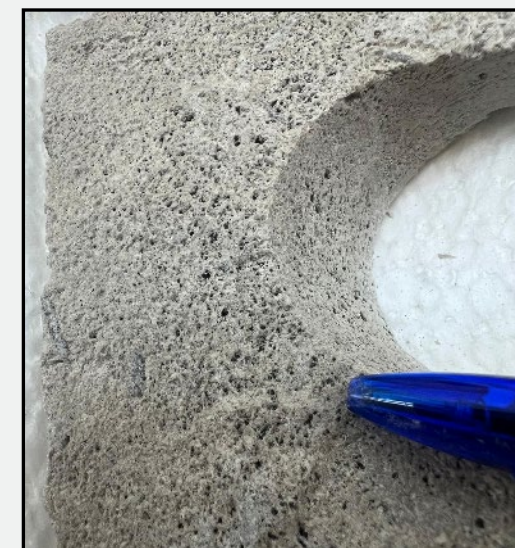
Kumli core with porosities over 25%
