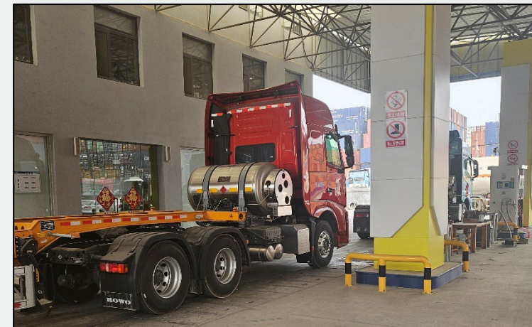
LNG fueled long haul transport trucks = 1250 km range
