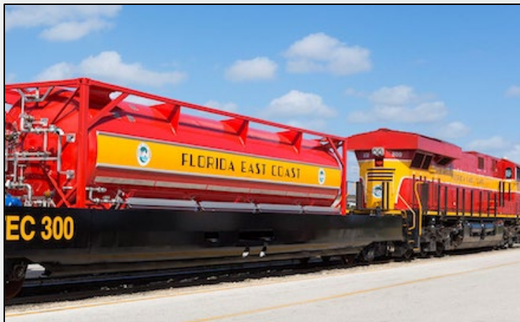
LNG increases locomotive operating ranges
