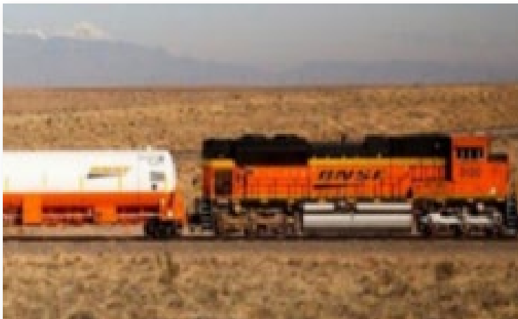
LNG increases locomotive operating ranges
