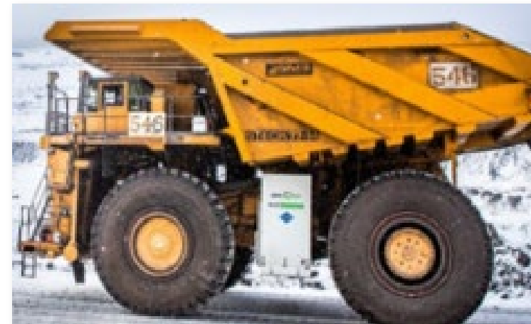
CAT has 10 MM hours using LNG as a dual fuel
