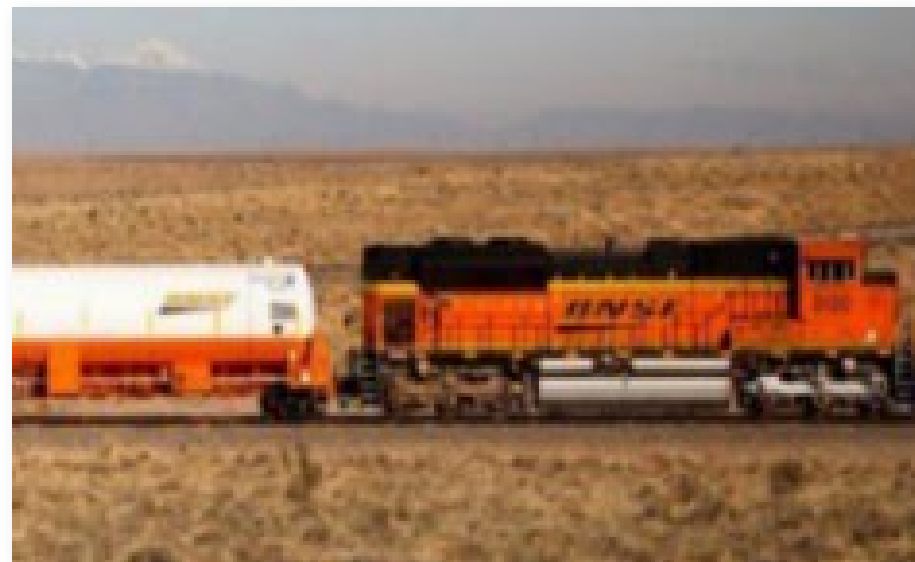
LNG increases locomotive operating ranges
