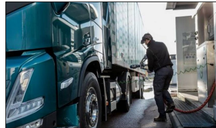
Refueling an LNG Long-Haul Transport Truck
