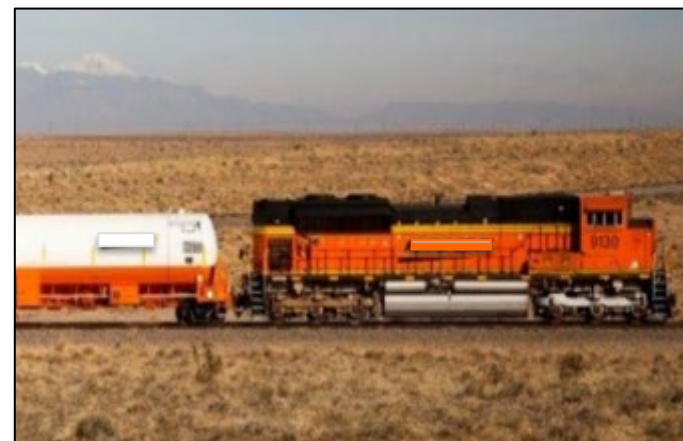
LNG Locomotive with Fuel Tender
