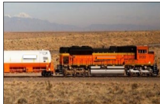
LNG Locomotive with Fuel Tender
